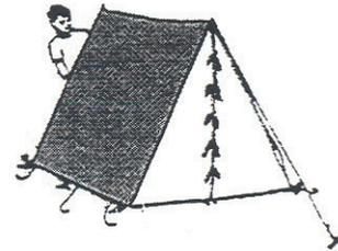
4. ASSEMBLE REAR TENT POLE, PUT IN PLACE. ATTACH REAR GUY LINE TO PEG AND PULL THE RIDGE TAUT.
